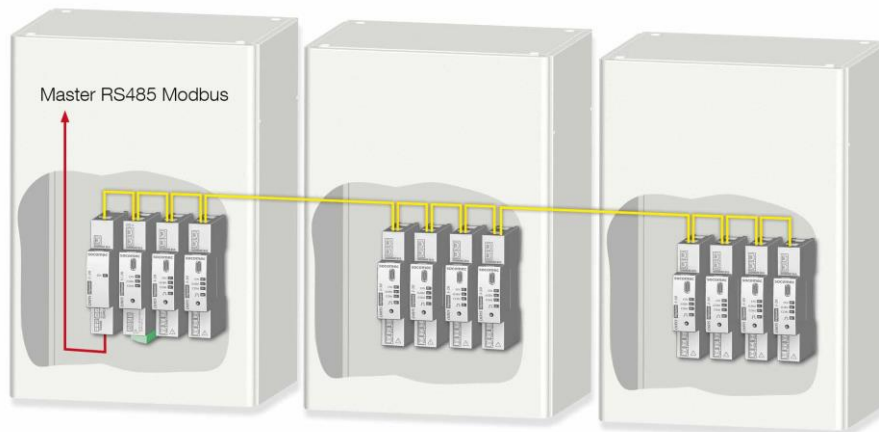
Fig. 7: Centralising on RS485 Modbus Supervisor – Cabinets in close proximity
