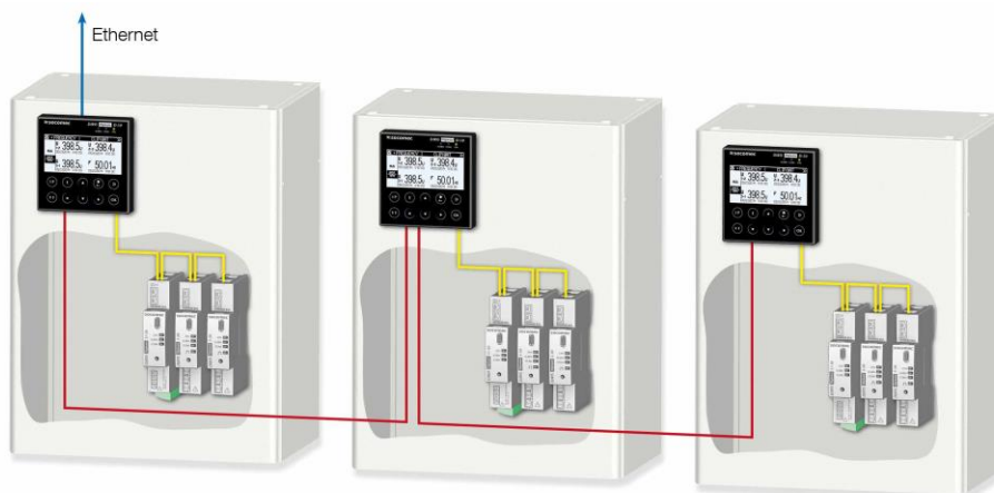
Fig. 14: Ethernet Supervisor and 3 separate Displays – Remote cabinets
